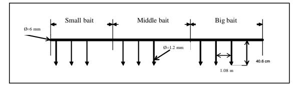
Figure 12: Longline arrangement for the experiment. Three lines with the bait sizes small (15 g), medium (25 g) and big were set in one skate.
