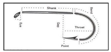
Figure 4: Basic parts of a J hook made of steel, coated with different metals (Bjordal and Løkkeborg 1996).
