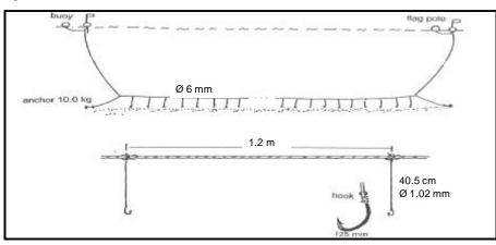
Figure 7: The whole view of a bottom set longline and hooking space. A mainline with a branch line carrying 500 hooks is set on the bottom by buoy and anchor (Hameed and Boopendranath 2000).
