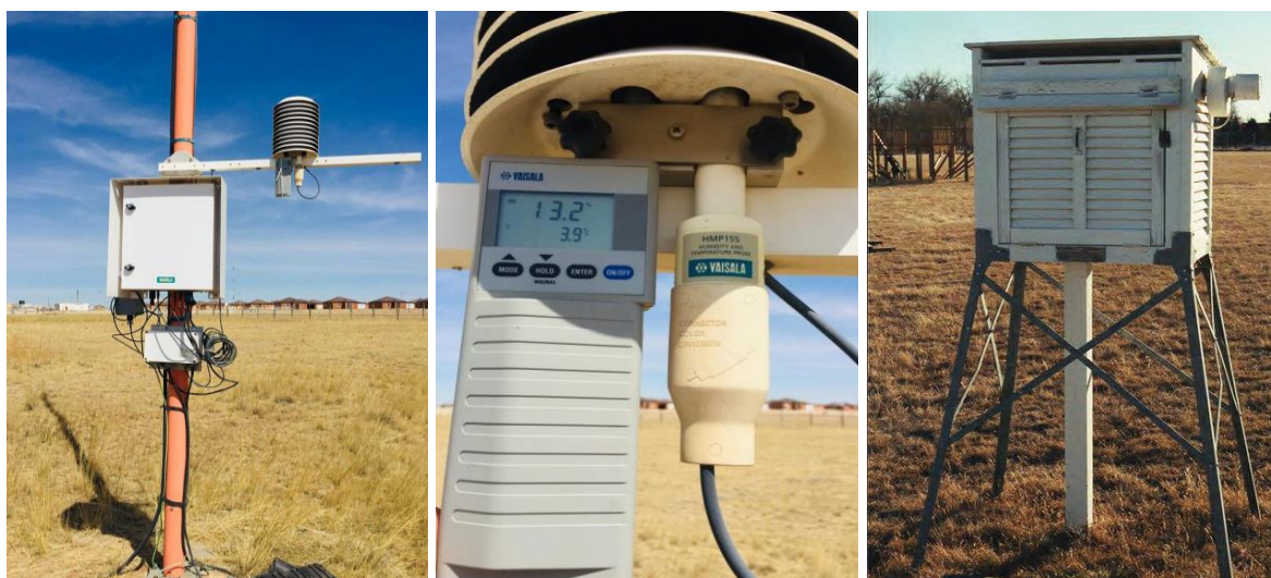
Figure 2. From left: MAWS301, the automatic weather station's data logger; an air temperature sensor (photos: G. Odbayar, B. Byambadorj, 2019); and a Stevenson screen (photos from Ryberg et al. 2009).
