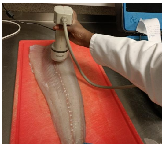
Figure 6. Taking colour measurements using a Minolta chroma meter CR-400
