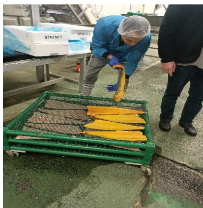
Figure 4. Arranging pollock fillets in drying racks
