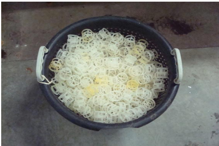
(b) Polypropylene bio ring for gas liquid interface in the aerator
