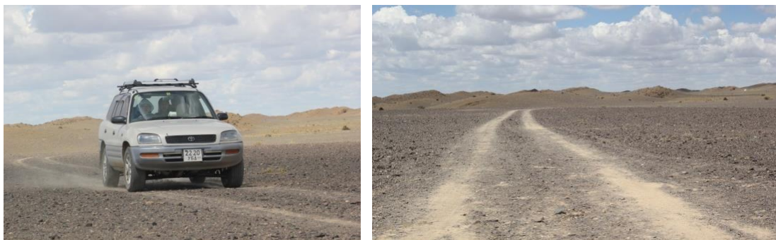
Figure 4. The off-road track simulation experiment. A 100-m stretch was driven 50 times to simulate the effect of typical off-road driving in southern Mongolia.
