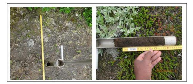
Figure 4. Soil sample taken 0.5 m from willow patch (left). Soil taken at 10 m depth by a soil auger (right). (Photos: K. Balikoowa, 29 June 2014).
