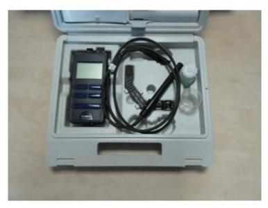
Figure 6. Conductivity meter used in this study (type: Cond 315i SET) produced by the German company Wissenschaftlich-Technische Werkstätten GmbH (WTW).
