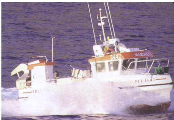
Figure 22: Single deck GRP high-speed fishing boat for longlining.
