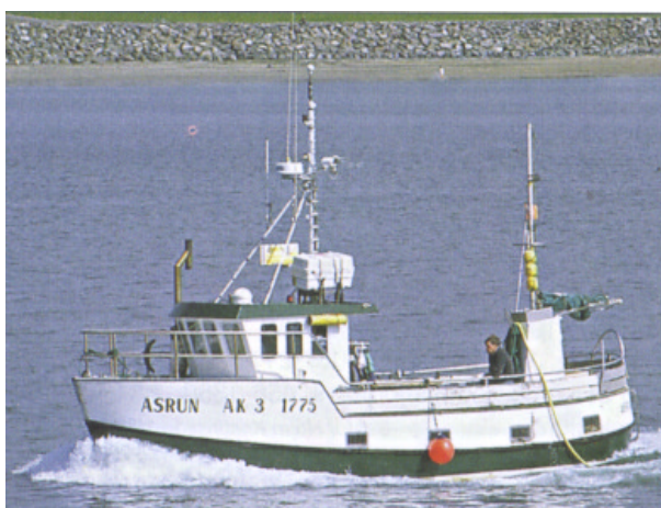
Figure 21: Single deck GRP fishing boat (displacement boat for gillnetting).
