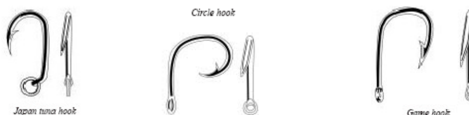
Figure 7: Hooks used for tuna and swordfish (Beverly et al. 2003).
