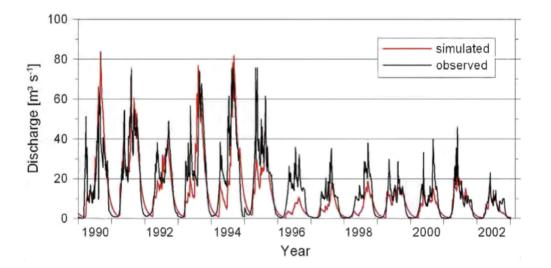
Fig. 10. Simulated and observed discharge of the River Kharaa near Darkhan (HBV-D Model) (Source: MOMO, 2009).
