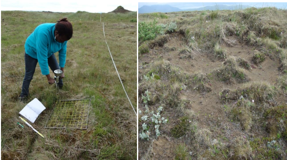
Fig. 9. Surface strength measured on the Upper Land (left). Erosion and pedestals on the Upper Land (right). (Photo: A. Balt, July 8 th 2011).
