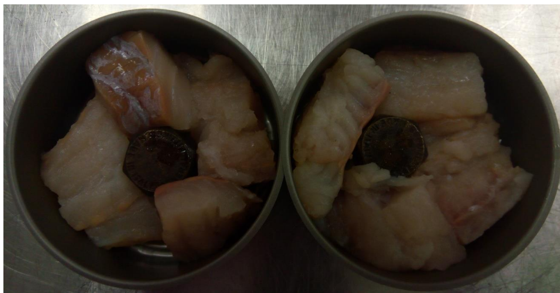
Figure 4. Heat loggers mounted in the centre of canned fish products
