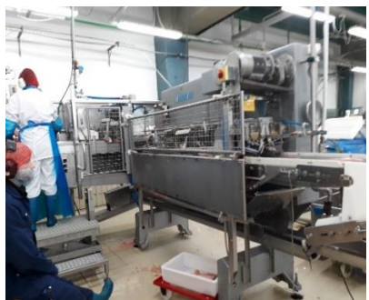
Baader gutting machine (153) in operation
