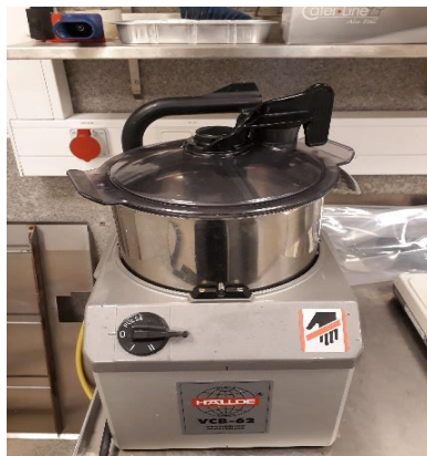
Electric mincer (VCB-62, Helde) used for mincing raw material
