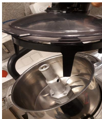
Inside view of electric mincer (VCB-62, Helde)
