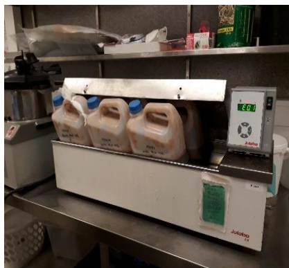
Silage containers in water bath at 45°C (Formic acid and Lactic acid))
