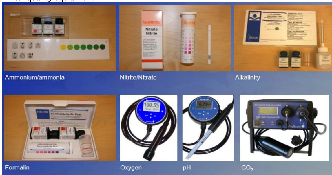
Figure 14: Equipments used for water quality measurement. Source : Billund aquaculture service (Aquatech, 2016).
