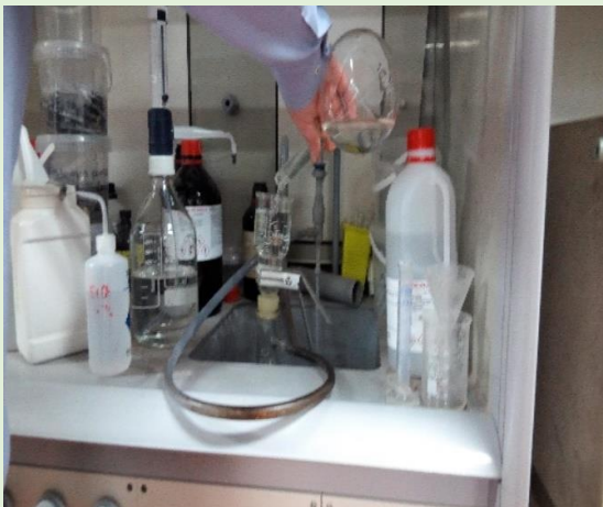
Filtrating a Litre of the sample H 2 O for TSS
