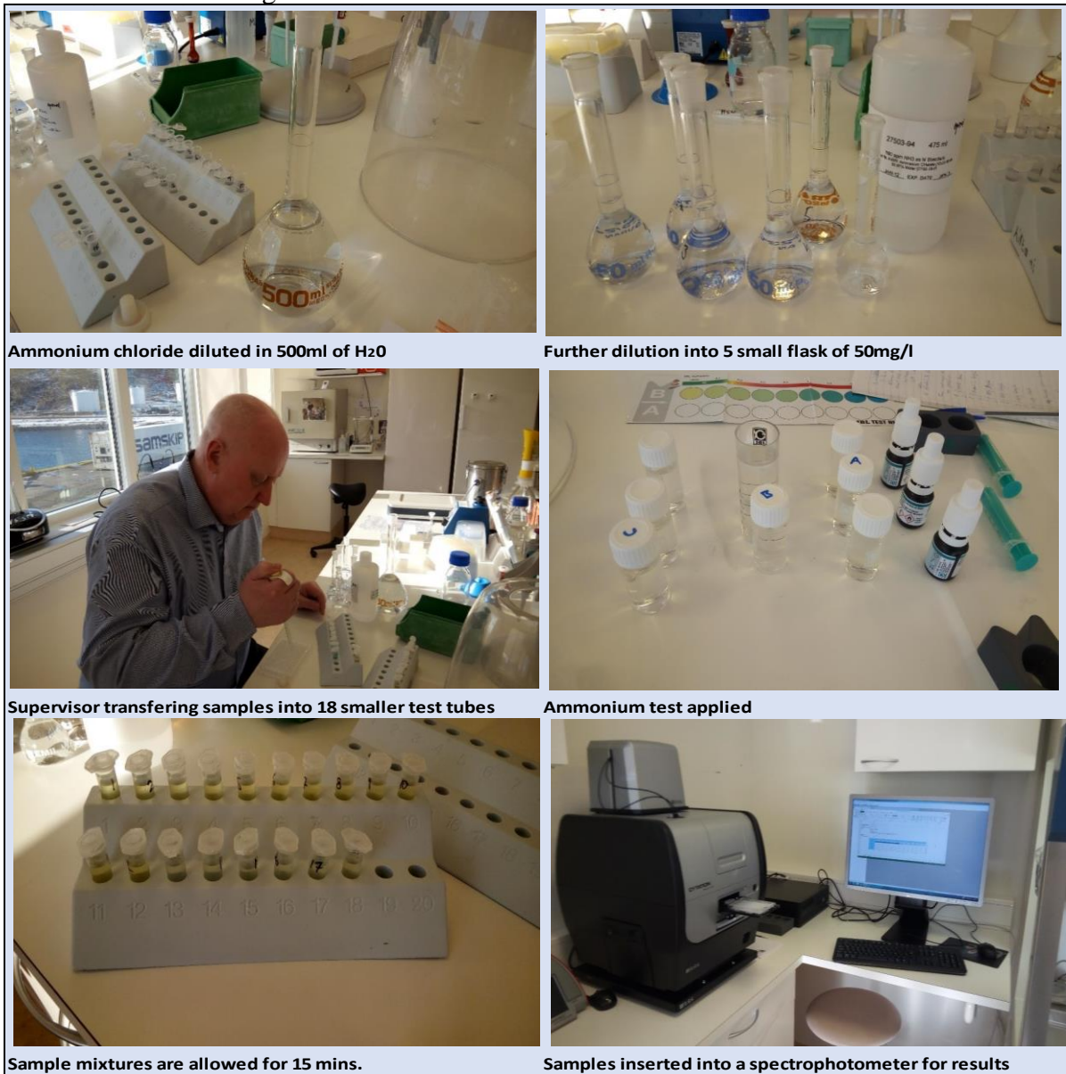
Figure 17: Measurement of total ammonium nitrogen (TAN).
