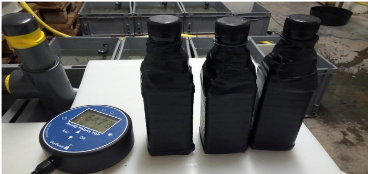
Figure 15: Measurement of Bacteria Oxygen Demand (BOD).
