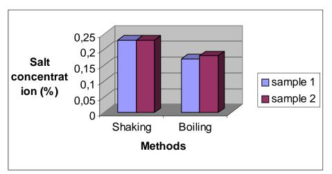
Figure 1. The difference between the shaking and boiling methods to determine sodium chloride by the volhard titration method in sample of light salted fillets haddock.
