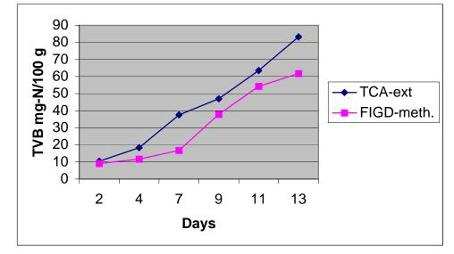
Figure 5. TVB analytical methods (TCA-extract, FIGD) used to determine freshness of herring that was stored at 0°C for up to 13 days.
