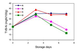
Figure 6: Development of TVB-N during storage of frozen-thawed shrimp dipped with sodium metabisulphite ( $Na_2S_2O_5$ ) and undipped, kept in ice and ice slurry.
