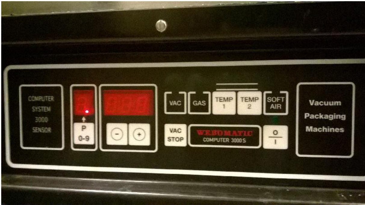
Figure 22: Control panel of vacuum packaging and gas flushing machine
