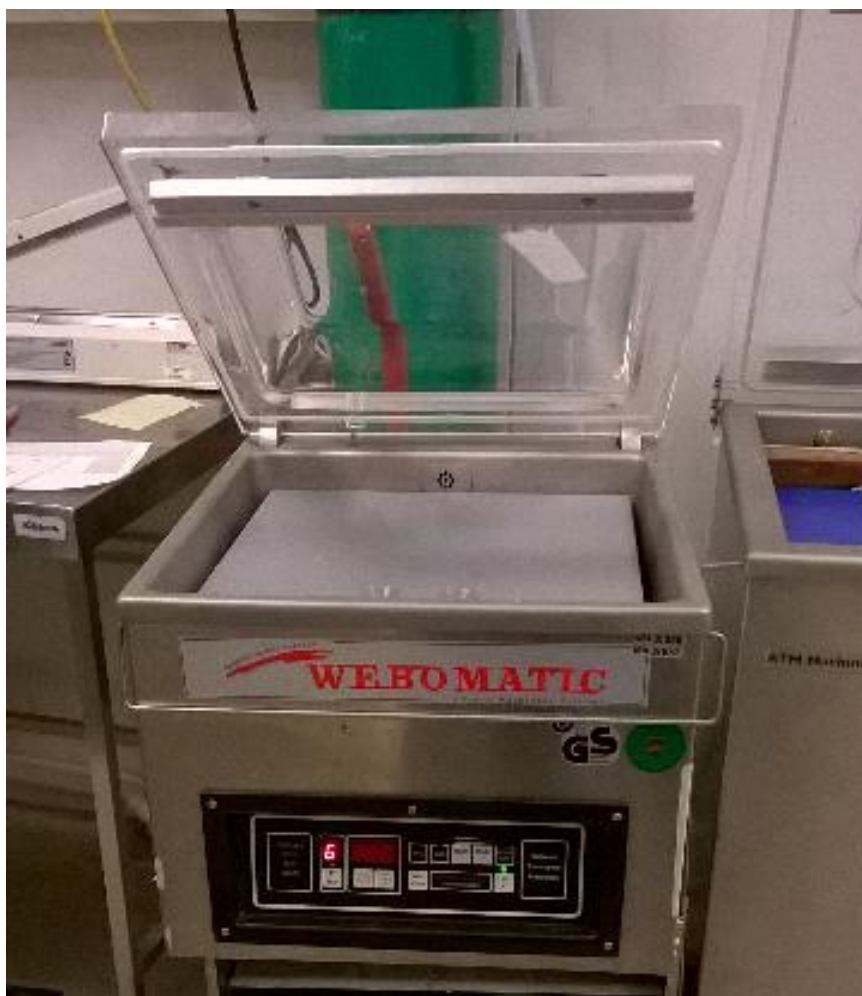
Figure 21: Webomatic vacuum packaging and gas flushing machine
