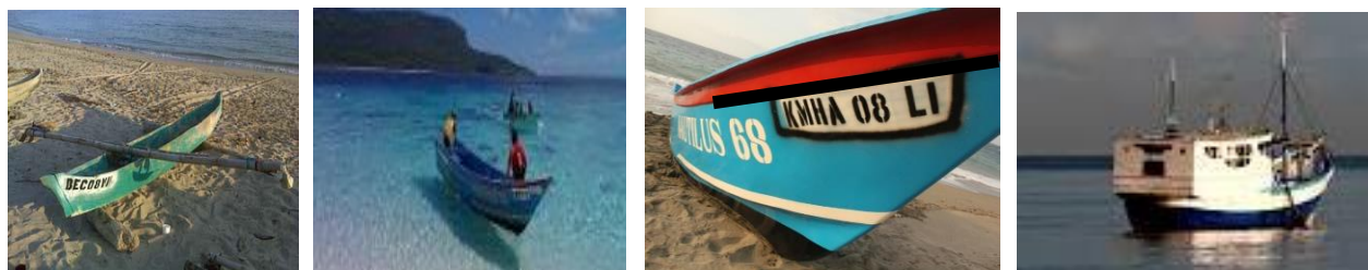
Figure 9: The shapes and size of boats used by small-scale fisheries, length 3-5 (left), 5-7 m (second from left), 7-9 m (third from left) and 10-12 m (right).
