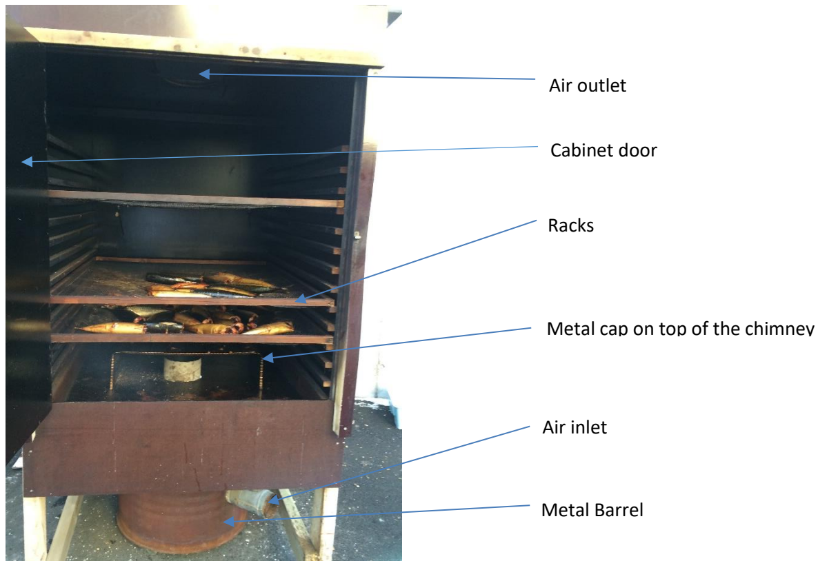
Figure 1: Hot smoking cabin main parts
