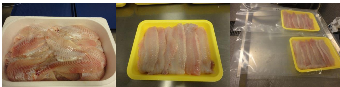
Figure 3: Deskinned redfish loins (left), loins laid in tray (middle) and trays in film bags ready for modified atmosphere packaging.
