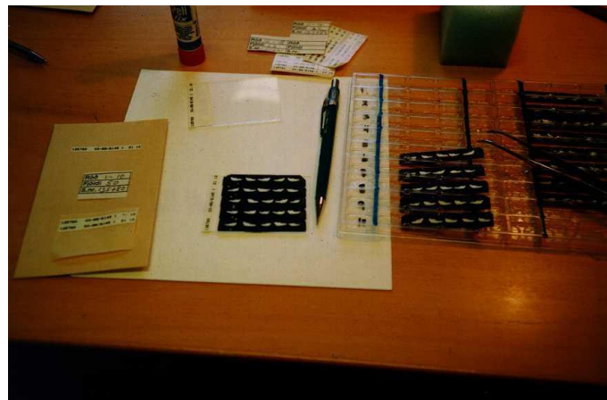
Figure 4. After the cutting of the black polyester resin block with 100 otoliths; the 20 sections of otoliths (5 x 20) are organized on 4 microscope slides; 25 otoliths in 5 rows on each microscope glass.
