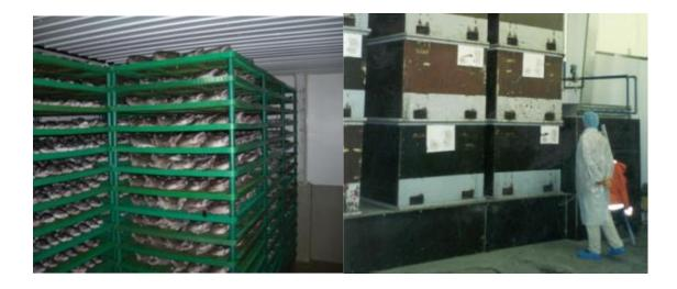
Figure 2: Fish heads on racks in the primary drying unit on the left and secondary air-drying unit with geothermal pipes on the right.
