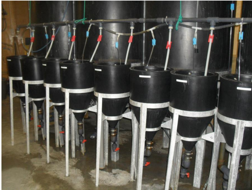
Figure 3: Rotifer silos used for the feeding trial experimental set up, with triplicate silos for each type of feed diet. The picture was taken by author at Staður in January 2014.
