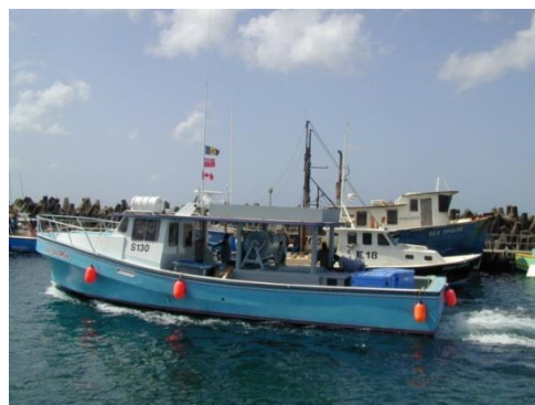
Ice Boat (GRP with integrated ice hold)
