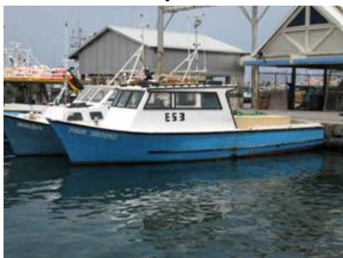
Ice Boat (Wood with detachable ice box)
