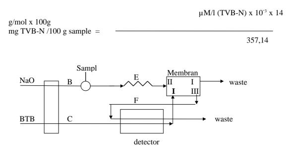
Figure 1: A schematic diagram of the Flow Injection/Gas Diffusion apparatus used for the determination of TVB-N.
