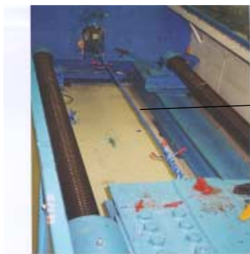
Figure 2: Tensile testing machine in the Hampidjan laboratory, used to measure breaking strength.
