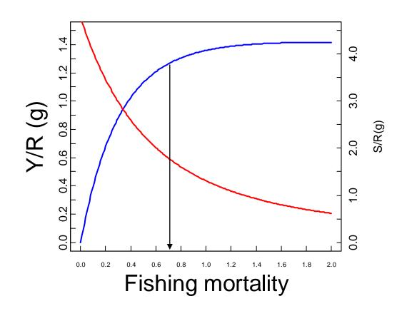
Figure 7: Yield per recruit and spawning stock per recruit curves for fishing mortalities ranging from 0 to 2. Arrow is showing fishing mortality corresponding to  $F_{0.1}$ .
