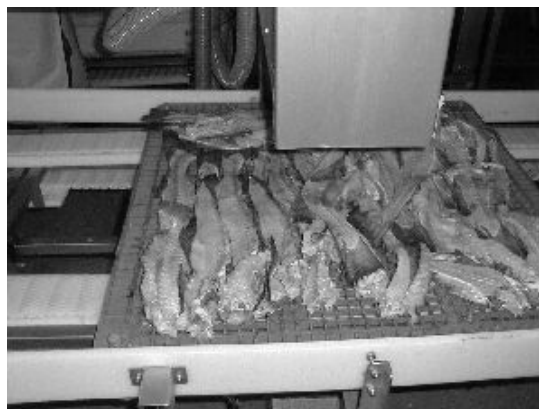
Figure 17: Backbones are ready to go into the drier at Laugafiskur Ltd.
