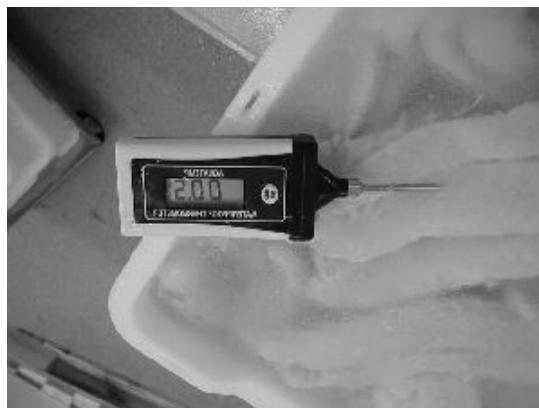
Figure 19: Temperature testing for a product sampled at the end of the processing line (H-039).
