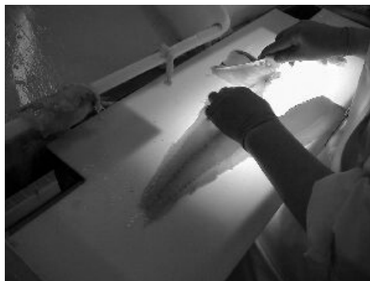
Figure 8: Trimming on the candle table in the plant (H-039).
