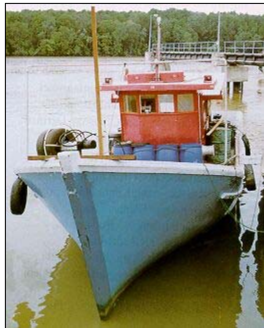
Figure 2: 12.75 m FRP boat built by MSB chosen as the standard design for a new Malaysian traditional boat.
