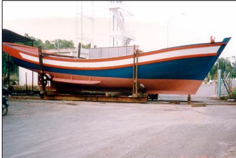
Figure 17: Hull of 15.85 m FRP boat built by MSB using the mould less technique after completion.
