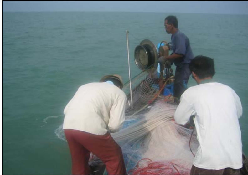
Figure 4: Picture of a locally-made net hauler, which is widely used among gillnetters in Malaysia.
