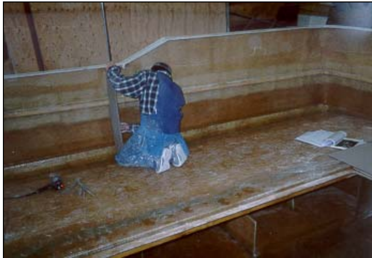
Figure 5: A worker at Seigla, boat building company in Iceland laminating the reinforcement of the hull.
