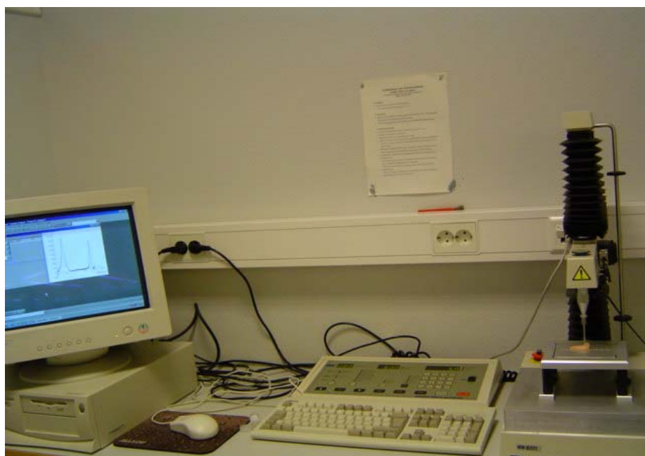
Figure 2: Texture analyzer (TA-XT2I Texture Analyzer) used to measure texture change in shrimp.
