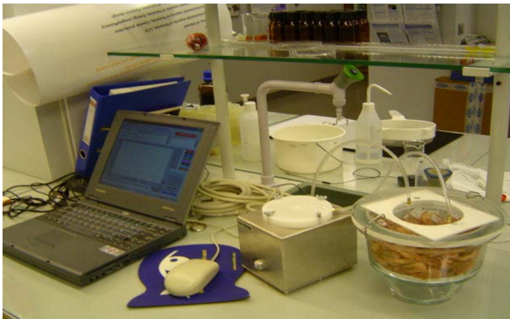
Figure 3: Electronic nose FreshSense used to measure quality change of shrimp.
