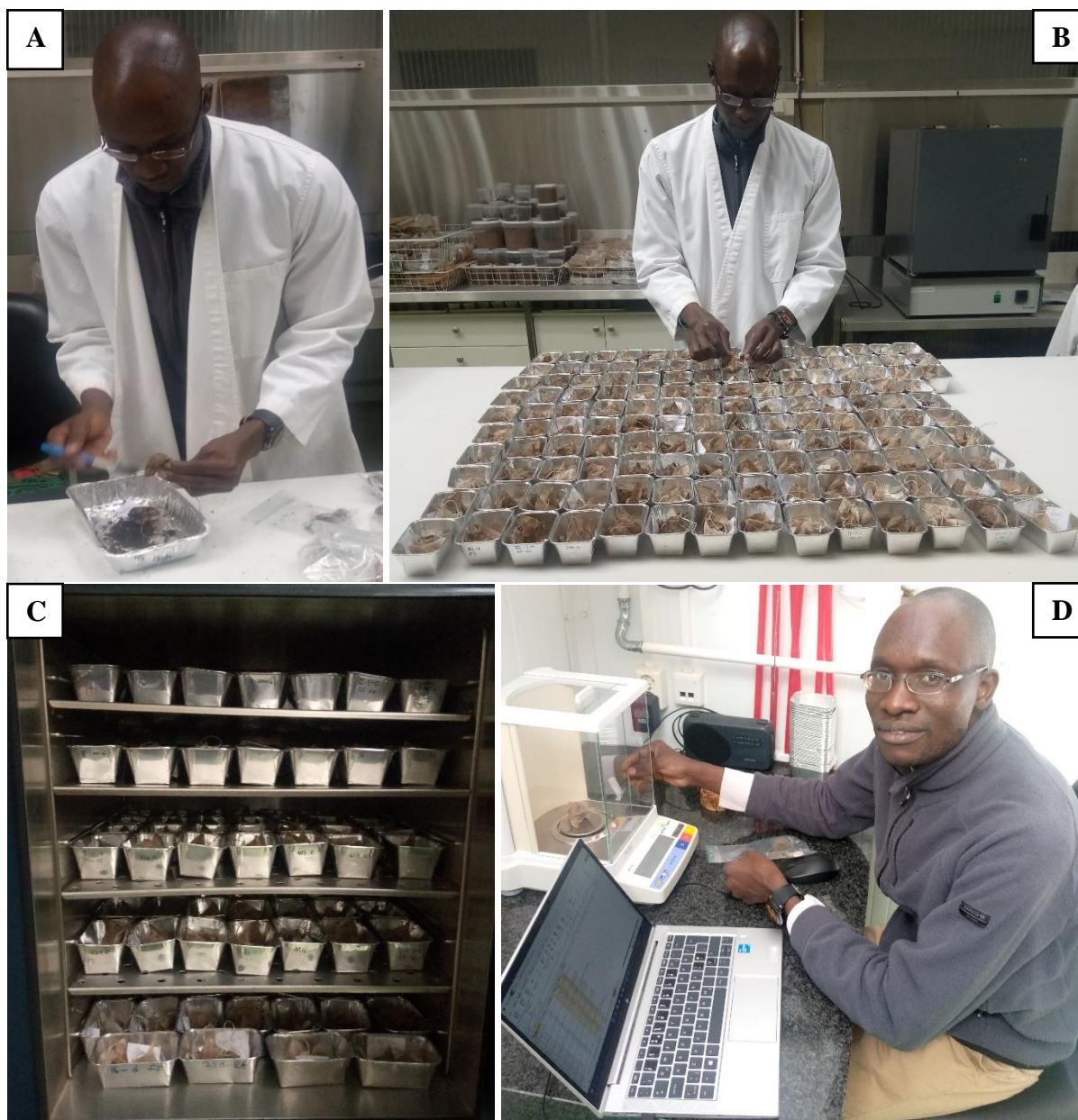
Figure 4. Showing the processes in the laboratory. (A) gentle cleaning of adhered soil particles and cutting of the roots that had entered the tea bags during incubation in the field, (B) tea bags were packed in pairs with a paper tag denoting their plot in small aluminium boxes, (C) boxes containing the tea bags were placed in an oven for 48 hours at 70°C, and (D) the tea bags were weighed and their weights recorded.
