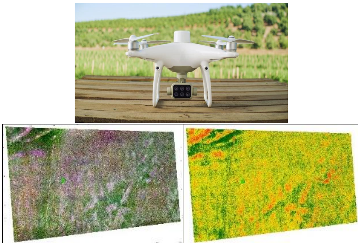
Figure 4. Multispectral aerial images and multispectral UAV used for aerial image acquisition: top) DJI P4M drone; bottom left) true colour RGB raster image, including all five bands; bottom right) NDVI raster image calculated using band 3 and band 5.
