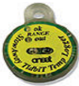
Figure 8: Onset logger used to record the surrounding temperature profile from Ný-Fiskur to F. S Pieters, Belgium.
