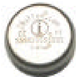
Figure 4: iButton logger used in the study to record the temperature of the loins placed in the polystyrene boxes.
