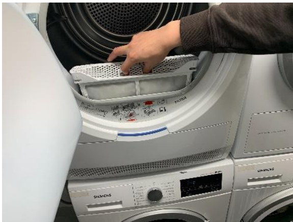
Figure 4 Loose fibre filter being removed from the dryer
