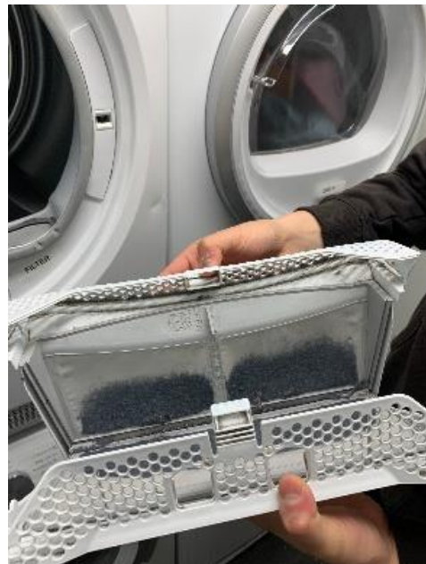
Figure 5 Loose fibres to be removed from the filter
